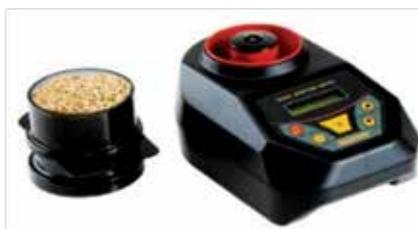
Monitor the moisture content of seeds using Moisture Meters (right) and the relative humidity inside the containers using humidity strips. Correlate seed moisture content with RH using Cromarty's equation<sup>2</sup>
